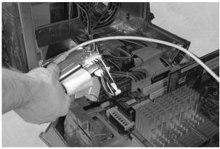
Attach the supplied IEEE 1394 cable to an internal FireWire  $\hspace{-0.8em}^{\tiny \textcircled{\tiny \$}}$  port in your system.
