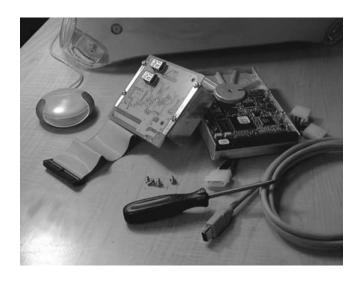
Attach the Lava IEEE 1394-IDE drive controller to your IDE hard drive with the four screws included in the kit.
