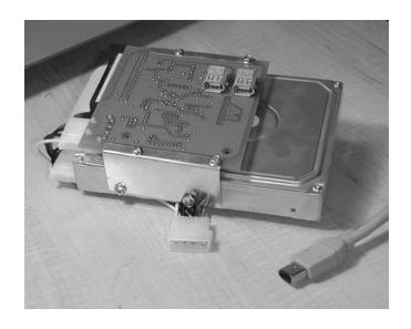
Slide the assembled unit into a drive expansion bay in your computer's chassis (Macintosh® G4 shown as an example).
