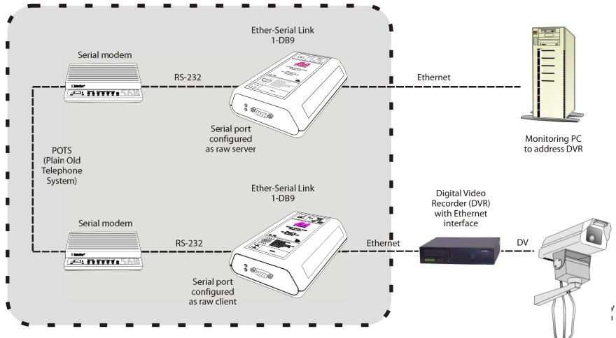
Shaded area is the equivalent of a null Ethernet cable of unrestricted length
