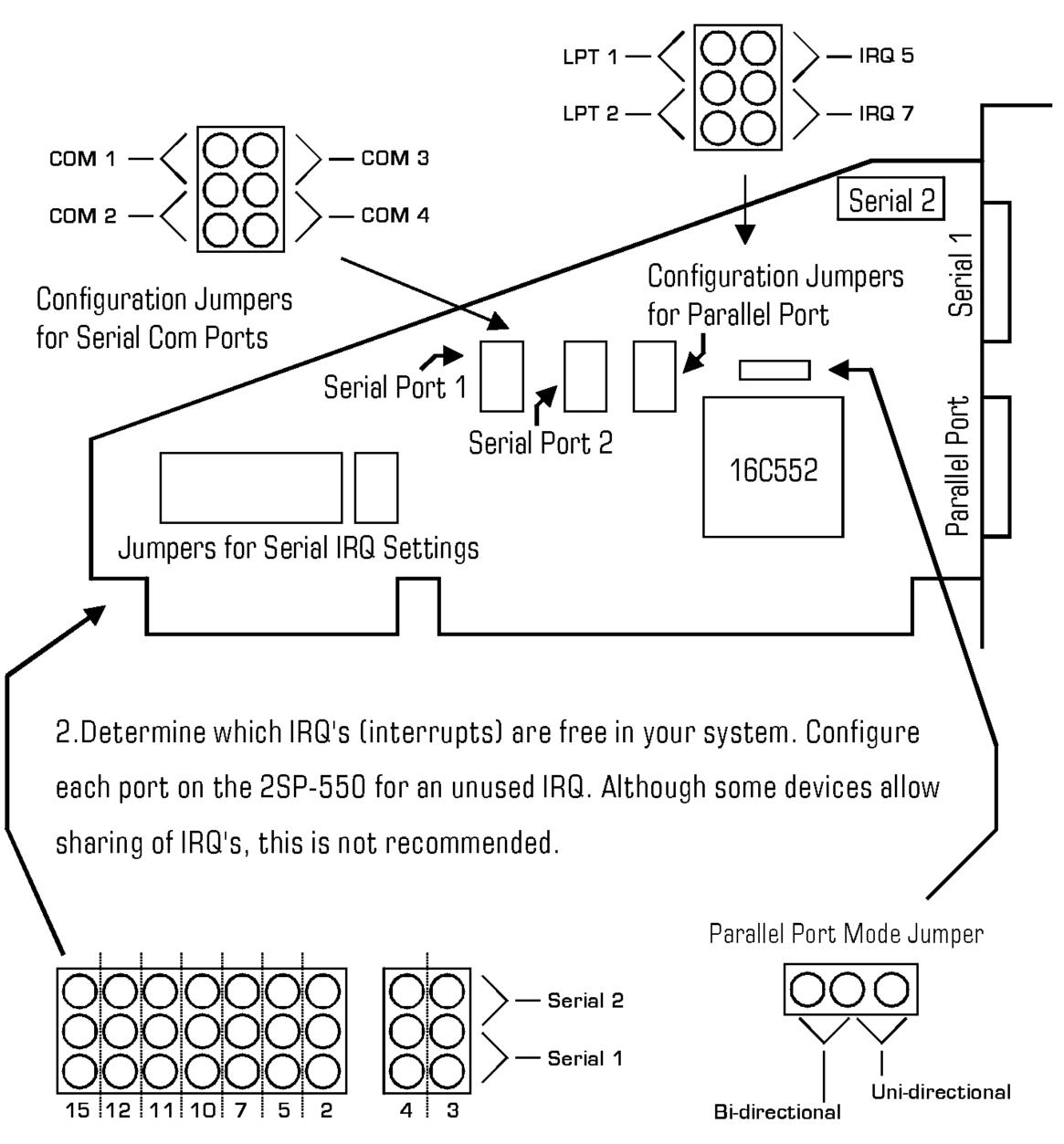
Note: To Disable a Port, remove the jumper from both of the corresponding COM or LPT <u>and</u> IRQ jumper configuration posts
