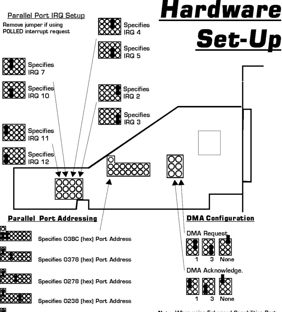
Note: When using O3BC (hex) address, O3BC ENABLE/DISABLE jumper must be ENABLED. When using all other addresses, O3BC ENABLE/DISABLE jumper must be DISABLED.
