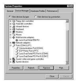
The DSerial-PCI hardware appears in Device Manager in two places: under the Multi-function adapters tree and as part of the Ports tree. Please note that any changes to the resources (I/O address and IRQ) used by either of the two ports on the DSerial-PCI must be made through the Resources page of the DSerial-PCI PARENT – not through the individual Ports pages.
