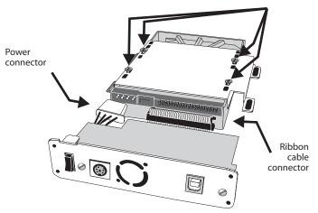
Firmly attach the power and ribbon cable connectors on the interface board to the hard disk drive.
