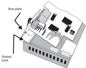
Fit the rear plate into the slotted tracks at the rear of the enclosure.
