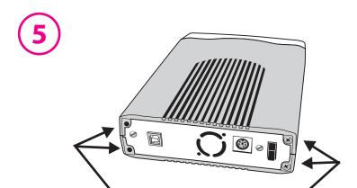
Secure the enclosure to the rear plate with four screws.
